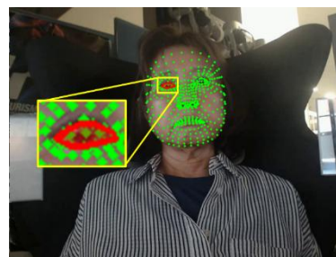
Fig. 2 Camera image and eye-area measurement using FaceMesh (Participant : Author)
