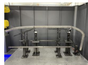
Fig. 1 Completed Hot Blow-Formed Pipe
