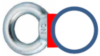
Eyebolt welding example
